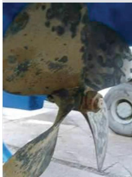
*Replacing the anodes would have been much cheaper than replacing this prop.*
