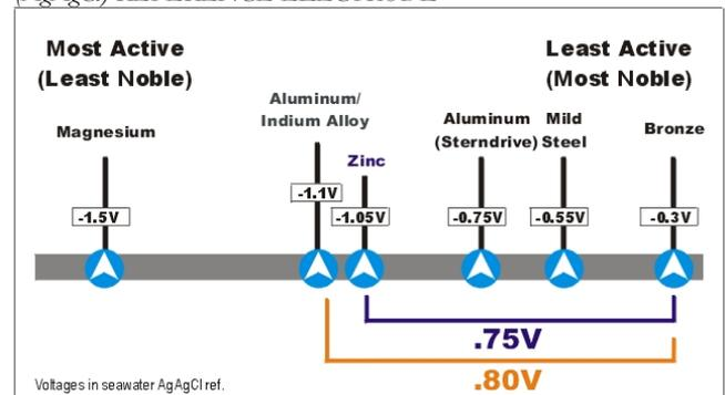
In order to provide protection, the highest practicable voltage difference possible is required between the sacrificial anode and the metal to be protected.
